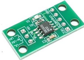
Gambar 4. Modul potensiometer digital X9C103S
