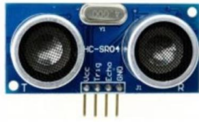
Gambar 3. Sensor ultrasonic HC-SR04
