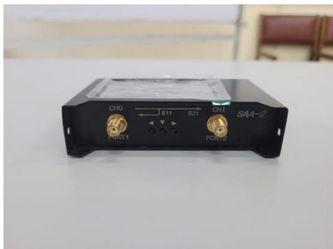
Gambar 6. Vector Network Analyzer - SAA2
