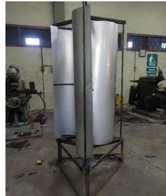
Gambar 8. Turbin angin savonius
