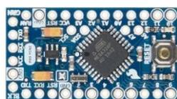
Gambar 1. Arduino Pro Mini
