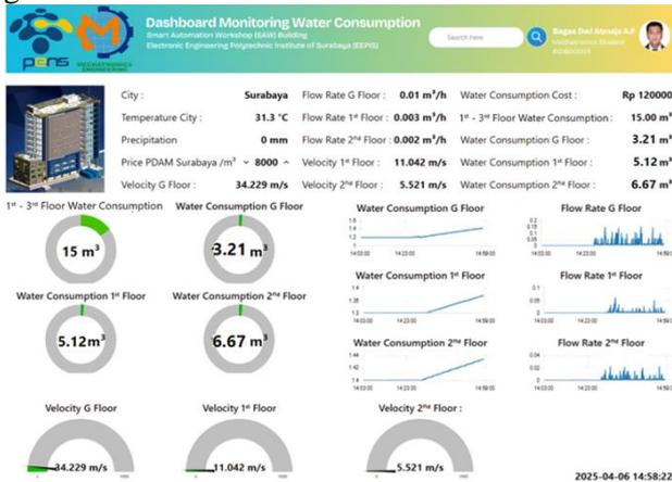
Gambar 10. Tampilan *Dashboard Monitoring* Pada *Platform Node-Red*
