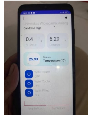
Gambar 11. Water Heater Off
