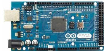
Gambar 2. Arduino Mega 2560
