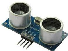
Gambar 6. Sensor Ultrasonik
