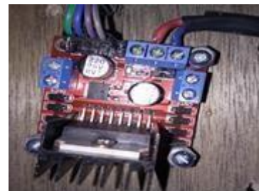
Gambar 2.4 Contoh Driver L298N(Sumber : Data Primer,2018)
