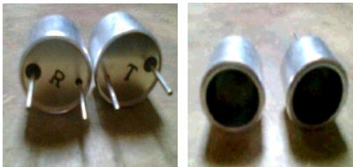
Gambar 2. Sensor Ultrasonik
