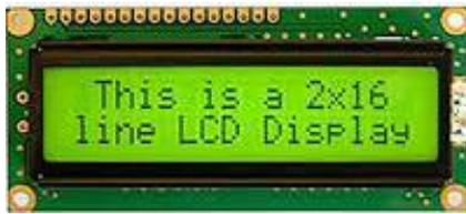
Gambar 6. LCD16x2
