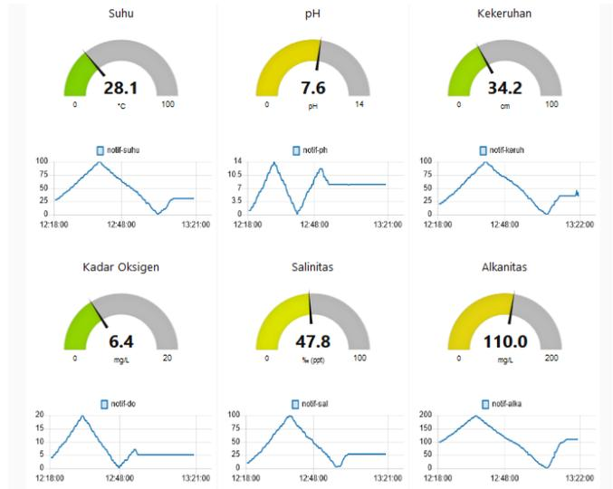
Gambar 13 Dashboard monitoring pengukuran
