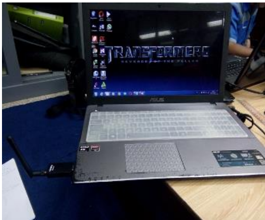
Gambar 4. 3DR Radio Telemetri Receiver ke port USB PC
