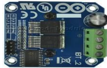
Gambar 7. BTS7960B 43A driver motor
