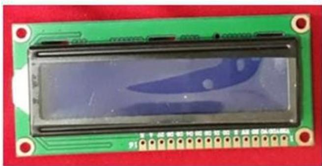
Gambar 1.3 LCD(Liquid Crystal Display)
